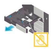
When loading envelopes of which the length is 7-3/16 inches (182 mm) or less, mount the Attachment on the Lateral Guide.
