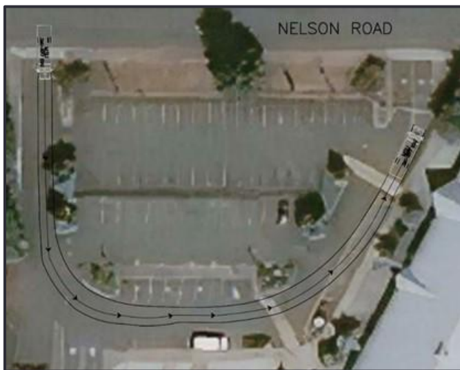
FIGURE 2. SHUTTLE BUS TURNING MOVEMENT
